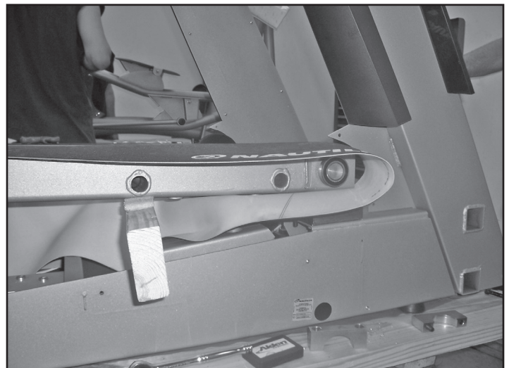
Figure 7: Lift treadle to create clearance.
